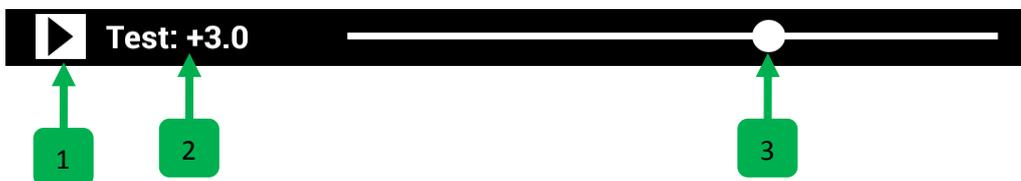
1. **Test icon**, pressing it will start or stop sounding our vario. It helps us to simulate the vario as if we were flying, and it will help us to choose better the values and adjustments that we like. When it is sounding, the sound of the vario will be updated dynamically as we change the values and settings.
